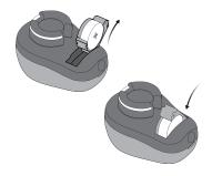
Open and close the battery drawer on the instrument(s), and place them close to your iPhone. The instrument(s) remains in pairing mode for 3 minutes.
