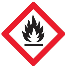
Safety sign to indicate flammable or highly flammable
